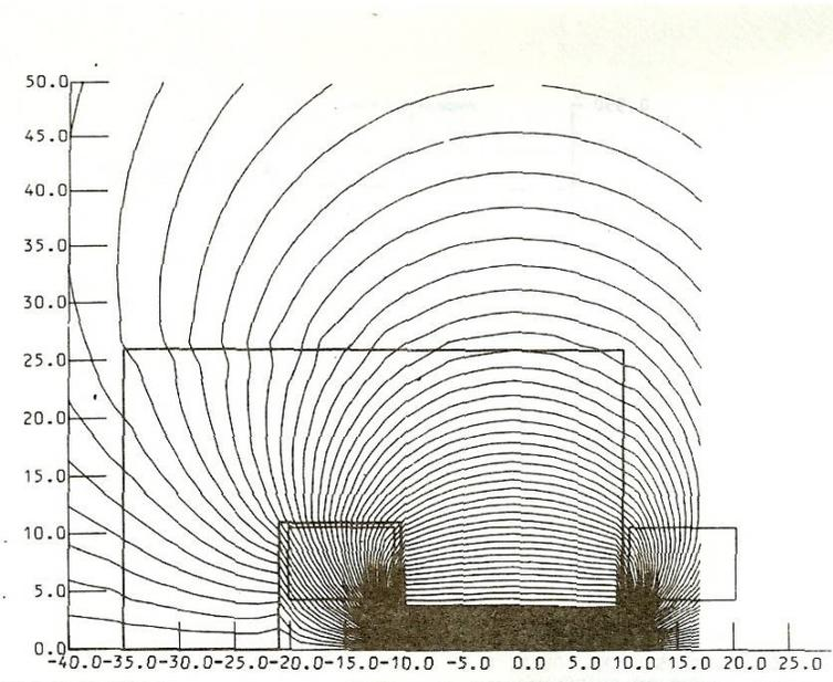
FIGURE 11 - A map of the computed magnetic scalar potential for a C-magnet
