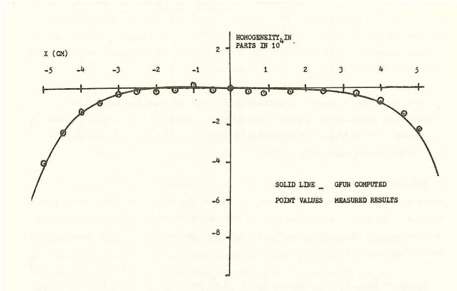
FIGURE 1 - Measured and computed homogeneity of the field produced by a c-shaped magnet with small pole tip shims
