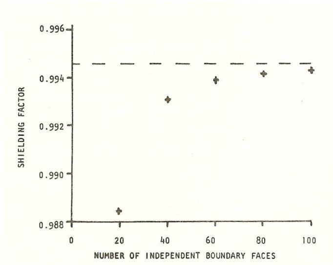
FIGURE 7 - Shielding factor of a hollow ferromagnetic cylinder – dimensions as figure 6, permeability 1000 - as a function of the number of independent boundary faces.
