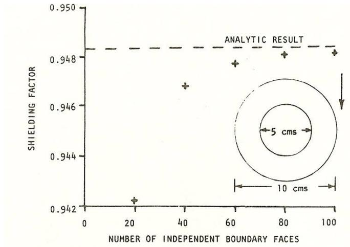
FIGURE 6 - Shielding factor of hollow ferromagnetic cylinder – Inside Radius 5 cm. Outside radius 10 cm. permeability 100 - as a function of the number of independent boundary faces in the model.
