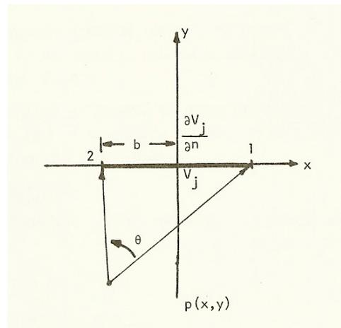
FIGURE 13 - Local coordinate system of an element
