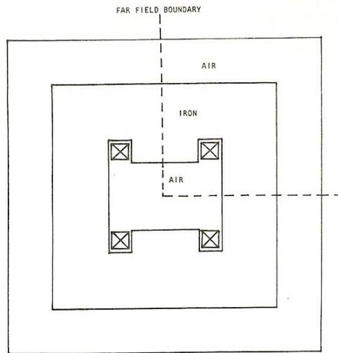
FIGURE 5 - Boundary integral method model using symmetry - the far field boundary is infinity
