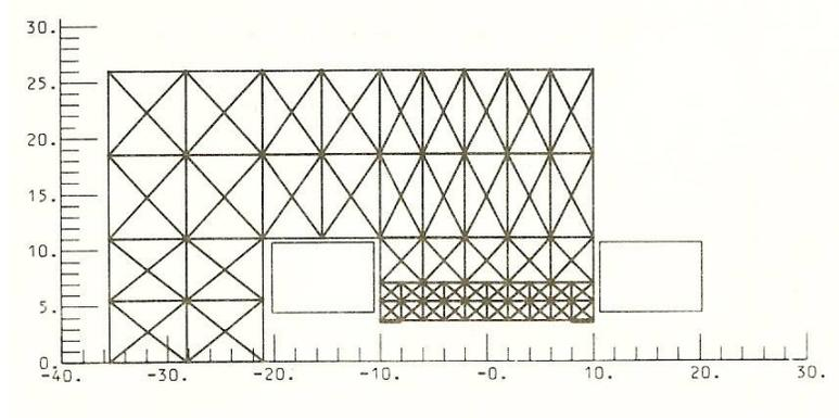
FIGURE 8 - GFUN Model of a two-dimensional C-magnet
