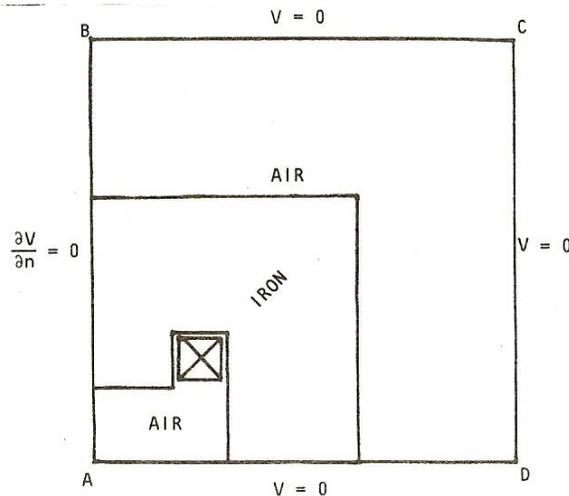
Figure 4 - Boundary integral method model using Neumann and Dirichlet boundary values
